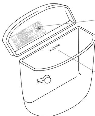
Part numbers are imprinted on the underside of the tank lid. Toilets manufactured prior to 1990 do not have part number labels on the underside of the lid.
