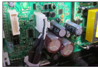
Figure 38 - Cable Wired to Board
