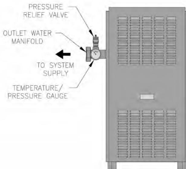
Figure 12: Supply Water Manifold Piping
