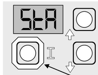
Press “I” key on the control to change from one parameter to the next. Each setting will alternate between display code (for example 5tA) and value.
