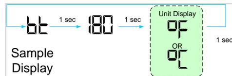
Please note that in operating mode to hold the display on the value the user can press and hold either the Up ↑ or Down ↓ keys and the value will be continuously shown. This may be helpful in watching a value “live”.
