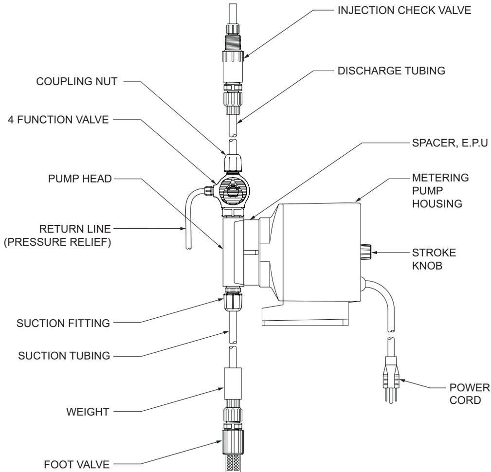
Metering Pump Component Diagram
