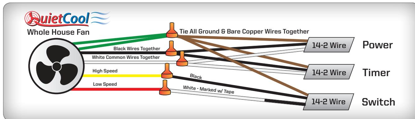
7. Begin wiring the fan by opening up the handy box. Take off the wire nuts within the handy box. Detach the green ground wire from the power cord. **Remove the power cord.** Re-attach the ground screw and wire to the handy box. Cut your green ground wire in half and strip both sides.
