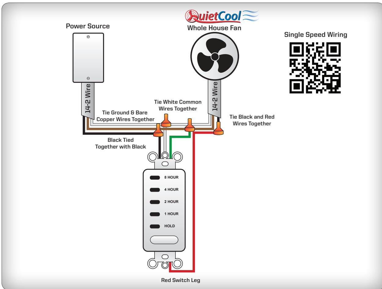
4. Using a wire nut, tie the white common wires from the Romex to the white common wire on the timer.
