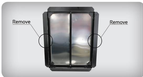
3. Using a flat head screwdriver, remove the two side flanges on the damper box. Make sure that you are removing the flanges on the same side as the flanges you removed on the vertical adapter. **(See Figure 2)**
