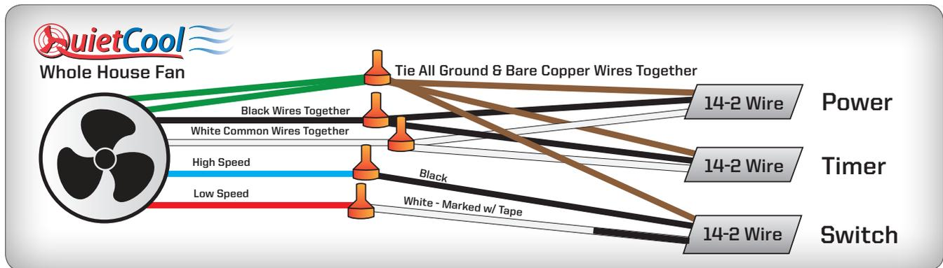
12. Begin wiring the fan by opening up the handy box. Take off the wire nuts within the handy box. Detach the green ground wire from the power cord. **Remove the power cord.** Re-attach the ground screw and wire to the handy box. Cut your green ground wire in half and strip both sides. **(see Figure E)**
