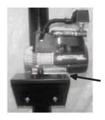
The compressor comes with male and female threaded rubber feet for mounting to the QL bracket. Install the rubber feet male (stud) part into the mounting bracket and the female part to secure the compressor. Use the remaining hardware (nuts, bolts and washers) to secure these feet to the bracket and the compressor.
