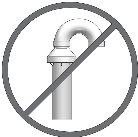
Figure 5-5 Do Not Install U-Bend to Rain Cap
