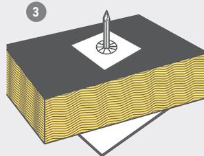
3 Secure with a self locking washer, included with Insulation Hangers
