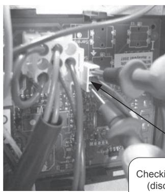
Checking continuity of sensor (disconnected at Control Board)
