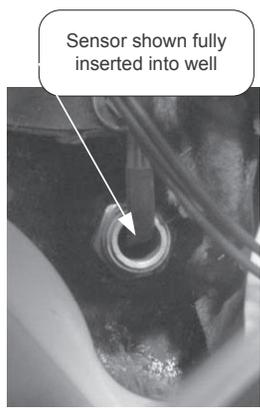
Sensor shown fully inserted into well
