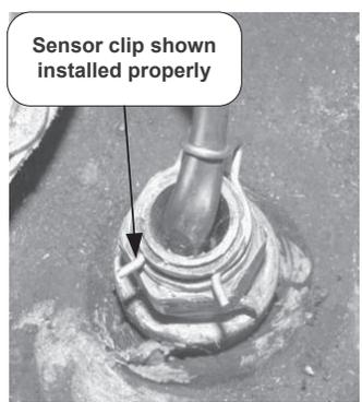
Sensor clip shown installed properly
