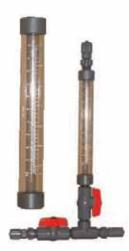
Calibration columns are used on the supply side of the pump to permit flow calibration. Never subject the column to vacuum or pressure. The calibration kits includes compression fittings for connecting them to pumps with tubing connections, and isolation valves. To determine the minimum column capacity (mL); Multiply the pumps' rated flow rate, GPH x draw down time,
