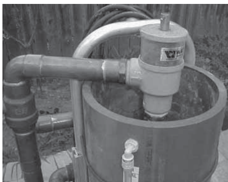
Figure 7a: Typical Cleanable Flush Cart Strainer (100 mesh [0.149mm])
