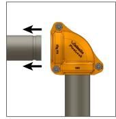
2. Loosen the nuts only on the outside and inside locations of the fitting end where the first mating component end is to be removed. Remove the mating component from the loosened side. Verify that the fitting is secured to the other mating component to prevent the fitting from
