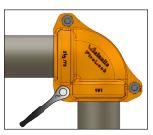
5a. COMPLETELY TIGHTEN NUT AT **INSIDE LOCATION:** Completely tighten the nut at the inside location until metal-to-metal contact occurs at the bolt pad. Verify that the fitting's keys engage the groove completely and that the oval neck of the bolt seats properly in the bolt hole.
