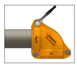
4a. TIGHTEN NUT AT OUTSIDE LOCATION: Tighten the outside nut at the corresponding location until metalto-metal contact occurs at the bolt pad. Verify that the fitting's keys engage the groove completely and that the oval neck of the bolt seats properly in the bolt hole.
