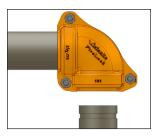
5. INSERT SECOND MATING **COMPONENT END:** Insert the second grooved mating component end into the other opening of the fitting. The grooved mating component end shall be inserted into the fitting until contact with the pipe stop of the gasket occurs. A visual check is required to verify that the fitting's keys align with the groove in the mating component end.
