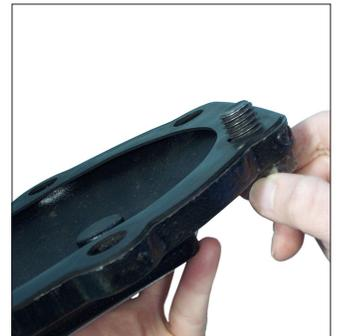
2. Align the holes of the cover plate gasket with the holes in the cover plate.
