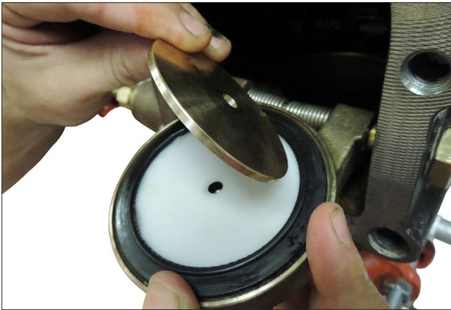
3. Remove the seal-retaining ring. Save the seal-retaining ring for re-installation.
