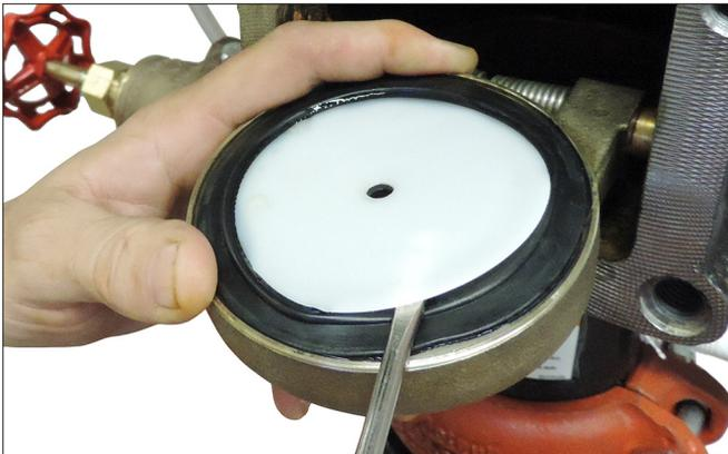
4. Pry the edge of the seal washer from inside the clapper seal, as shown above. **DO NOT PRY THE SEAL WASHER OUT FROM THE INNER HOLE.**
