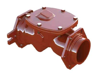
A removable Top Cover allows easy maintenance to the Patriot II<sup>TM</sup> Security Check Valve when needed. Clow's Security Check Valve has an MJ x Stab end connection and can be installed on any 6" mechanical Joint Connection, ensuring compatibility with all hydrant brands and providing the flexibility and cost effectiveness you demand.
