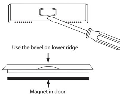
Gently slide a screwdriver into the bottom edge of the badge. Gently turn the screwdriver counter clockwise. The badge is held on by a magnet in the well of the battery door. The badge should pry off easily. **DO NOT USE FORCE.**
