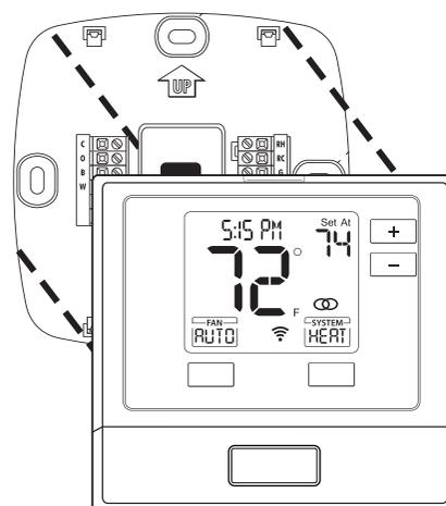
Align the 4 tabs on the subbase with corresponding slots on the back of the thermostat, then push gently until the thermostat snaps in place.
