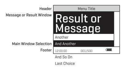
As described previously, the volume button allows an exit or escape from the current menu and a return to the previous menu. This allows a rapid exit from an inner menu to the main menu by repeatedly pushing the volume button. Pushing at any time will turn the colorimeter off.
