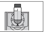
6. Remove tube from colorimeter.
