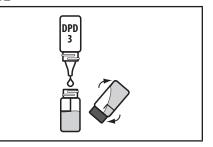
NOTE: For wastewater samples, <u>Standard Methods for the Examination of Water and Wastewater</u> recommends waiting 2 minutes for full color development when testing total chlorine.
