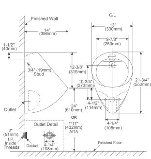
\*\*Recommended for ADA height installation for 17" floor to rim.
