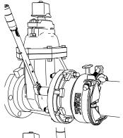
**Step 6** • Bring the mating flange into position and assemble the flange joint using the flange bolts. Be sure to maintain proper pipe insertion described in Step 4.
