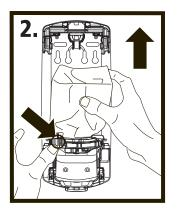
If removing used refill, push latch to release refill. Remove refill and dispose. See recycling instructions below.
