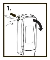
Open dispenser by pushing on one of the dual side latches until it releases and pull down on front cover.
