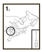
Using a flat-head screwdriver, remove collar and cap on refill bottle and discard.
