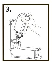
Push refill pump down into pump house, ensuring collar snaps into place.
