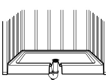
**14 Install the end walls. Engage the end wall pins in the back wall slots.**
