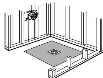
**9 Connect the drain to the drain pipe. Position a protective liner in the basin.**
