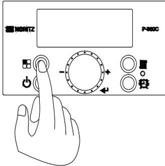
1. Turn off the power to the control panel. Press and hold the 'Function Button' for approximately 5 seconds to get into the 'Installer Mode'.
