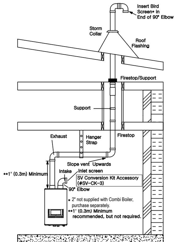
**■ Provide adequate combustion air so as to not create negative pressure within the building.**
