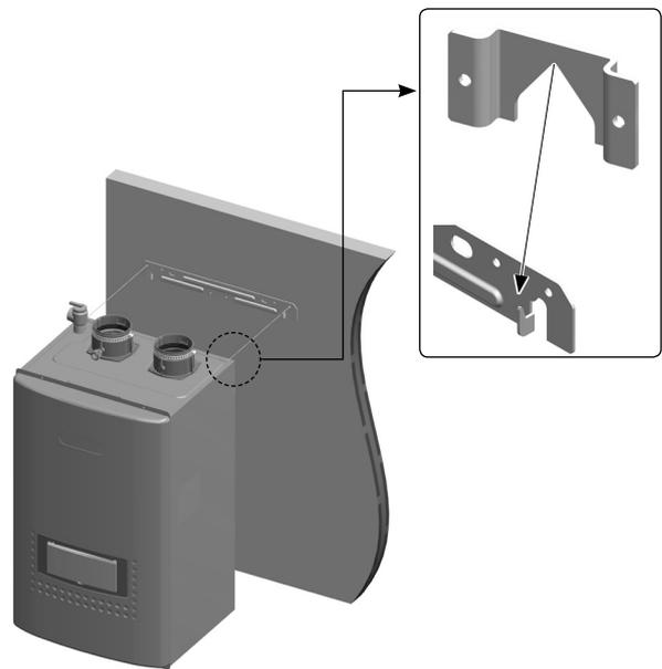
6. Locate the lower mounting bracket on the bottom of the Combi Boiler. The two screws and dry wall anchors will be used to secure the bottom of the unit to the wall.
