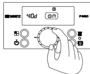
14. Press the 'Dial Button'. The default setting of ON will begin to flash on the display. Turn the 'Dial Button' to OFF if desired.
