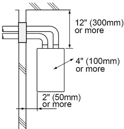
**Securing of space for repair/inspection**
