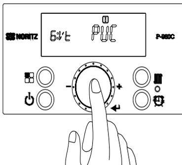
4. Press the 'Dial Button' ('PVC' will be blinking), then turn the 'Dial Button' clockwise so 'CPVC' is blinking.
