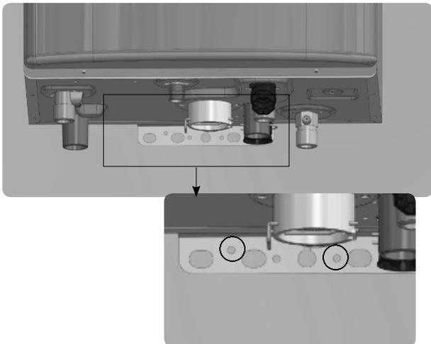
7. Mark two holes. Then remove the Combi Boiler from the wall.
