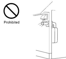
Before installing, make sure that the exhaust flue termination meets clearance requirements proper clearances according to the National Fuel Gas Code (ANSI Z223.1).
