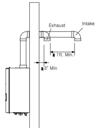
**Vent Pipe Installation (SV-Non Direct Vent)**
