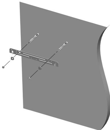
5. Lift up the Combi Boiler, rest the unit on the hooks provided on the wall bracket that is already mounted on the wall.
