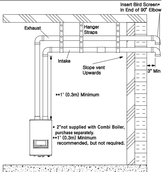
When choosing intake and exhaust terminations, you must use the same type of elbow (i.e. both 90° elbows). This will help with proper combustion by putting both terminations in the same pressure zone.
