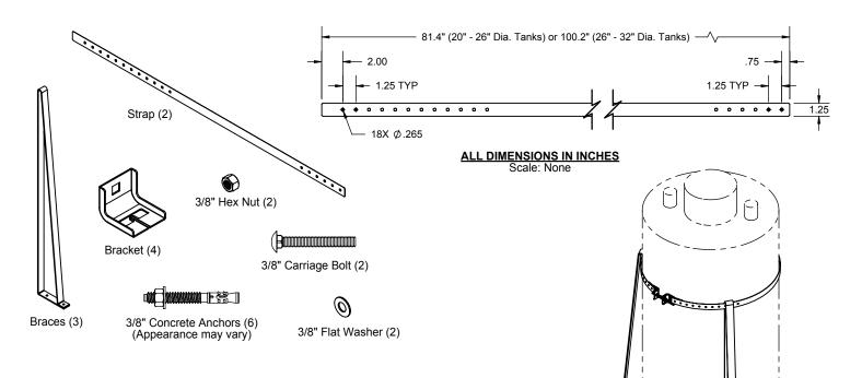
The HOLDRITE® Floor Mounted Water Heater Equipment Support is ideal for water heaters in open areas mounted directly to the floor. These floor mounted supports are certified to meet building code equipment anchorage requirements. For water heaters up to 100 gallons.
