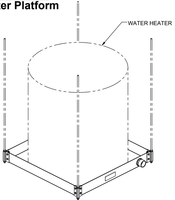
The #60-SWHP-A Suspended Water Heater Platform is engineered to support water heaters up to 50 U.S. gallons, or other equipment, up to 750 pounds total weight. This time and labor savings tool is designed for the Professional Contractor. Design features requested by plumbers are incorporated into a professional platform and drain pan combination that can be suspended with 3/8" or 1/2" all thread rods. See Installation Instructions for detail.
