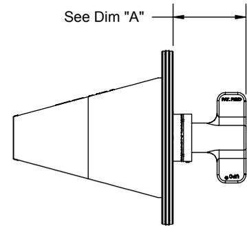
The TESTRITE® TRW2 through TRW6 (TEST WEDGES) are used in conjunction with TESTRITE TEE'S, which allow temporary blocking of the DWV stack for testing. Available in 2", 3", 4" & 6".
