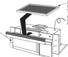
Filter Kit JX81H— Recirculating Charcoal Filter Kit To be used when the microwave oven cannot be vented to the outside.
