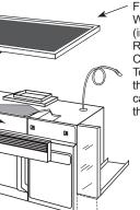
Filter Kit WB02X35607 (included) Recirculating Charcoal Filter Kit To be used when the microwave oven cannot be vented to the outside.
