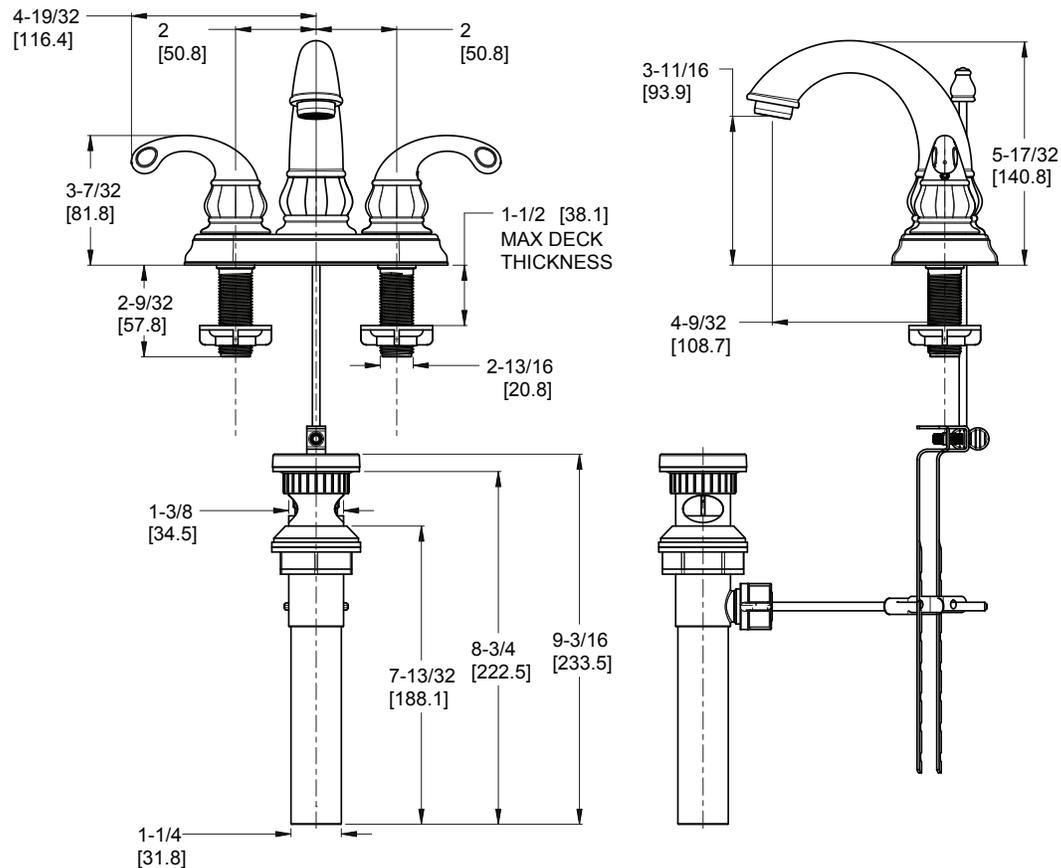
Ø1 Min to Ø1/2 Max. Deck Hole Openings
