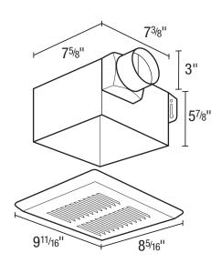
Acceptable for use over tub or shower when installed in a GFCI protected branch circuit.
