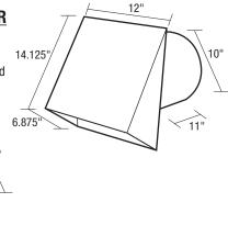
Fits 8" round duct Backdraft damper 22 gauge, galvanized steel construction
