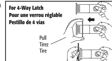
**CONVERTING 2-3/4" TO 2-3/8"(70mm TO 60mm BACKSET**
