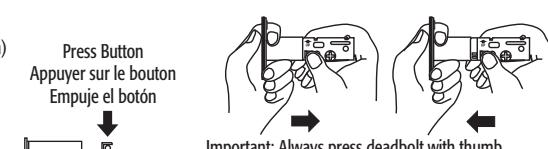
**CONVERTING 2-3/8" TO 2-3/4"(60mm TO 70mm BACKSET**
