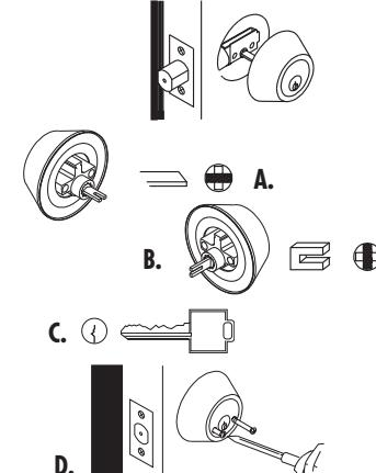
**BACKSET DEADBOLT ADJUSTMENT (This backset adjustment instruction applies only when adjustment is necessary.)**
