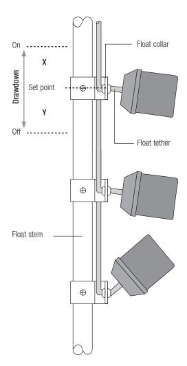
The "On" and "Off" positions describe normally open floats. For normally closed floats, the functions are reversed.
