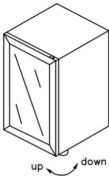
It is important for the beverage cooler to be leveled in order to work properly. It can be raised or lowered by rotating the plastic sheaths around each of the feet on the bottom of the machine. If you find that the surface is not level, rotate the feet until the beverage cooler becomes level. You may need to make several adjustments to level it. We recommend using a carpenter's level to check the machine.
