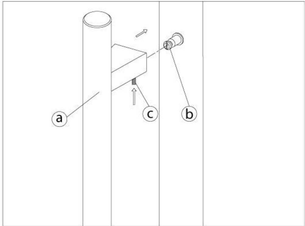
Place the handle over the fixing pin(s) of the door. Using the supplied allen wrench, tighten the grub screw(s) to secure the handle.
