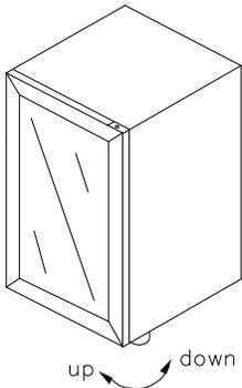
It is important for the wine cooler to be leveled in order to work properly. It can be raised or lowered by rotating the plastic sheaths around each of the feet on the bottom of the machine. If you find that the surface is not level, rotate the feet until the wine cooler becomes level. You may need to make several adjustments to level it. We recommend using a carpenter's level to check the machine.
