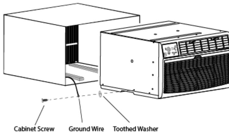
3. Gently slide the air conditioner cabinet into the Wall Sleeve. With the cabinet screw hole still exposed, attach the ground wire to the cabinet using the cabinet screw making sure that the Toothed Grounding Screw Washer is pressed against the cabinet.
