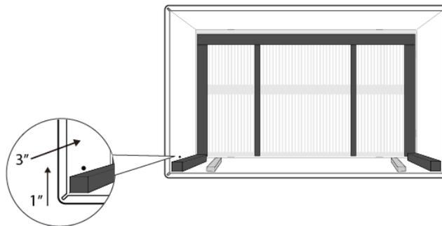
3. Attach one end of ground wire using 1 (one) Toothed Washer and 1 (one) Grounding Screw.
