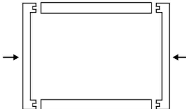
3. Pull the power cord through the Trim Kit frame and then slide the Trim Kit Frame over the unit until it is flush with the wall.
