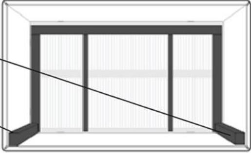
5. Attach 2 (two) - 1" X 1" X 17" Tapered Support Blocks as indicated. *Note: The tapered support blocks are sloped from 1" at the front down to 3/4" on the back. Please attach accordingly to allow for the unit to have a slight rearward slant when installed. This will help ensure proper drainage.*
