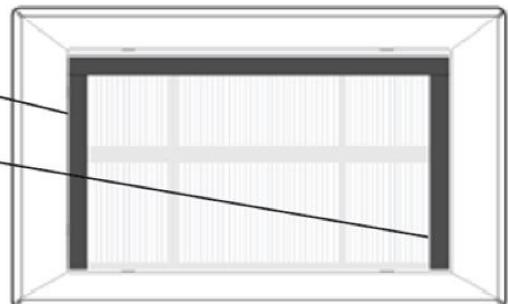
3. Attach 2 (two) - 1" X 3/4" X 14" Vertical Insulation Seals as indicated. (Attach 4 1/2" from left side and 4" from right side.)
