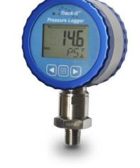
Data Loggers can be ordered in various ranges (see back for details). The logger is packaged in a rugged submersible anodized aluminum and stainless steel housing and has a standard 1/4" NPT fitting (1/2" NPT for 8700 and 14500 ranges). The replaceable internal lithium battery has up to a 3-year life.
