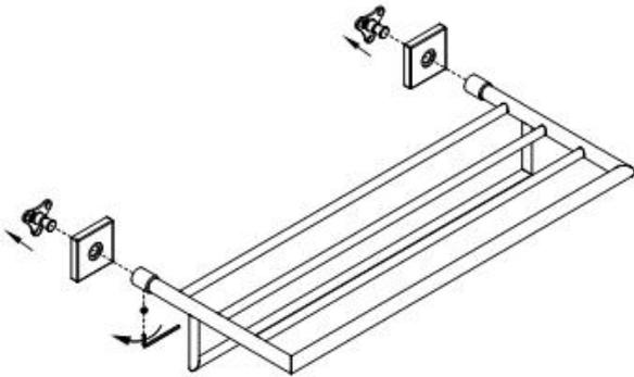
② ALIGN MOUNTING BRACKETS AND MARK LOCATION
