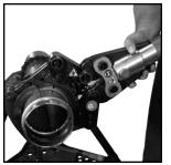
8. Squeeze adapter jaw arms to open the jaw. Rollers must be fully retracted to open the adapter jaw. Place the open adapter jaw into grooves in the pressing chain and let go of the jaw arms. Make sure the tube is inserted to the proper depth in the fitting (reference mark from #5). With the pressing tool perpendicular to the tube, begin the pressing cycle by pulling the trigger of the tool.
