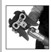
7. Release the pin (push and twist) on the jaw holder of the pressing tool, and install the adapter jaw on the tool. Return the pin to its original position, securing the jaw. The red sleeve on the tool must be in the back position to allow for crimping sizes 2½", 3" and 4". The red sleeve in the forward position allows for use with ½" - 2" standard pressing jaws.
