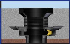
After concrete pour is complete, remove the temporary cap with pliers or water meter key as shown on the label. The cap eliminates the need for duct tape or other protective coating on the cover or strainer. The strainer spuds or the cleanout spuds are installed after the pour.
