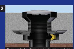
The concrete should be poured so that it is level to the top of the LevelBest adapter. The cap of the LevelBest allows the slab to be finished easily without using a hand trowel.
