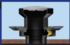
Set drain with LevelBest rough-in adapter at concrete pour level. The height can be adjusted by tightening or loosening the adapter.
