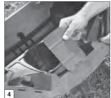
4 Install splash plate.
