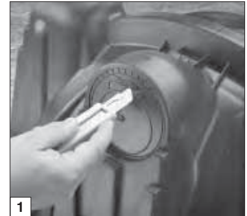
1 Start tear-out seal.
