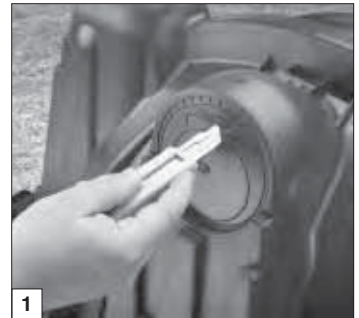
Start tear-out seal.
