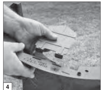
Install splash plate.
