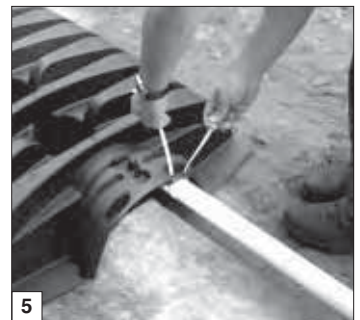
Secure pressure pipe.
