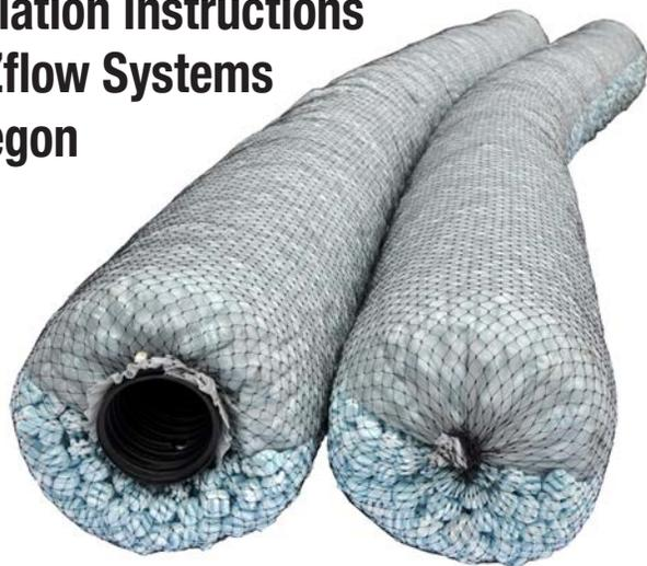
6. Place EZflow bundle(s) in the EZflow configuration per permit. The top or center-most bundles containing pipe are joined end to end with an internal pipe coupler. Any additional aggregate only bundles, should be butted against the other aggregate-only bundles and do not require any type of connection.
