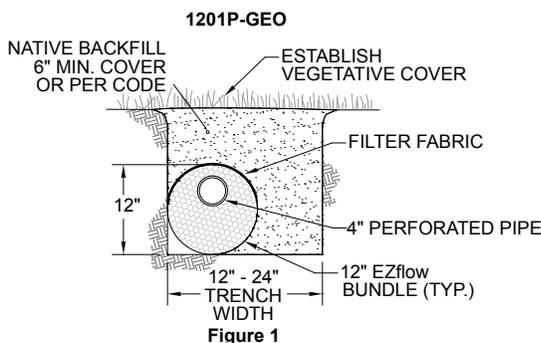
D. EZflow 1201P will be sized at the same required linear foot sizing for standard 2-foot wide gravel trench. For example, if the sizing for a 2-foot gravel trench requires 100-linear feet of trench, the 1201P system will be sized at 100-linear feet.
