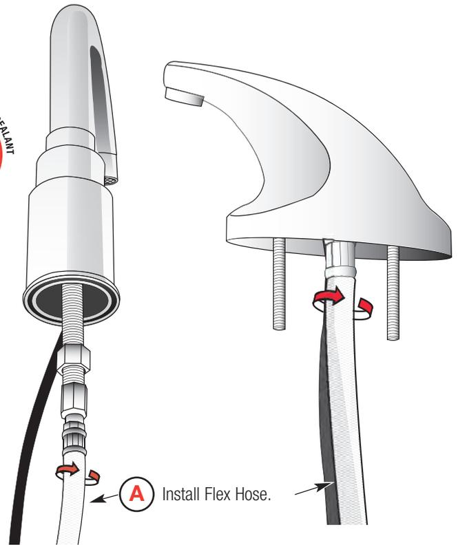
**2A - SF-2100/2150, SF-2200/2250, & SF-2400/2450 SERIES: INSTALL SPOUT, TRIM PLATE AND SPACER**
