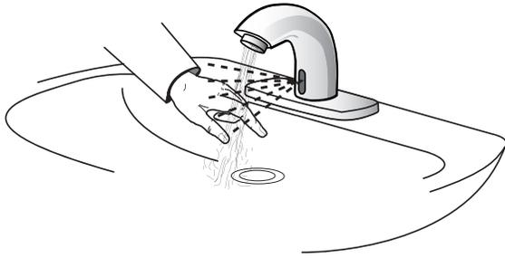
1. Place hands under faucet. Solenoid valve should “click,” LED in sensor window should blink once and water should flow from the spout.
