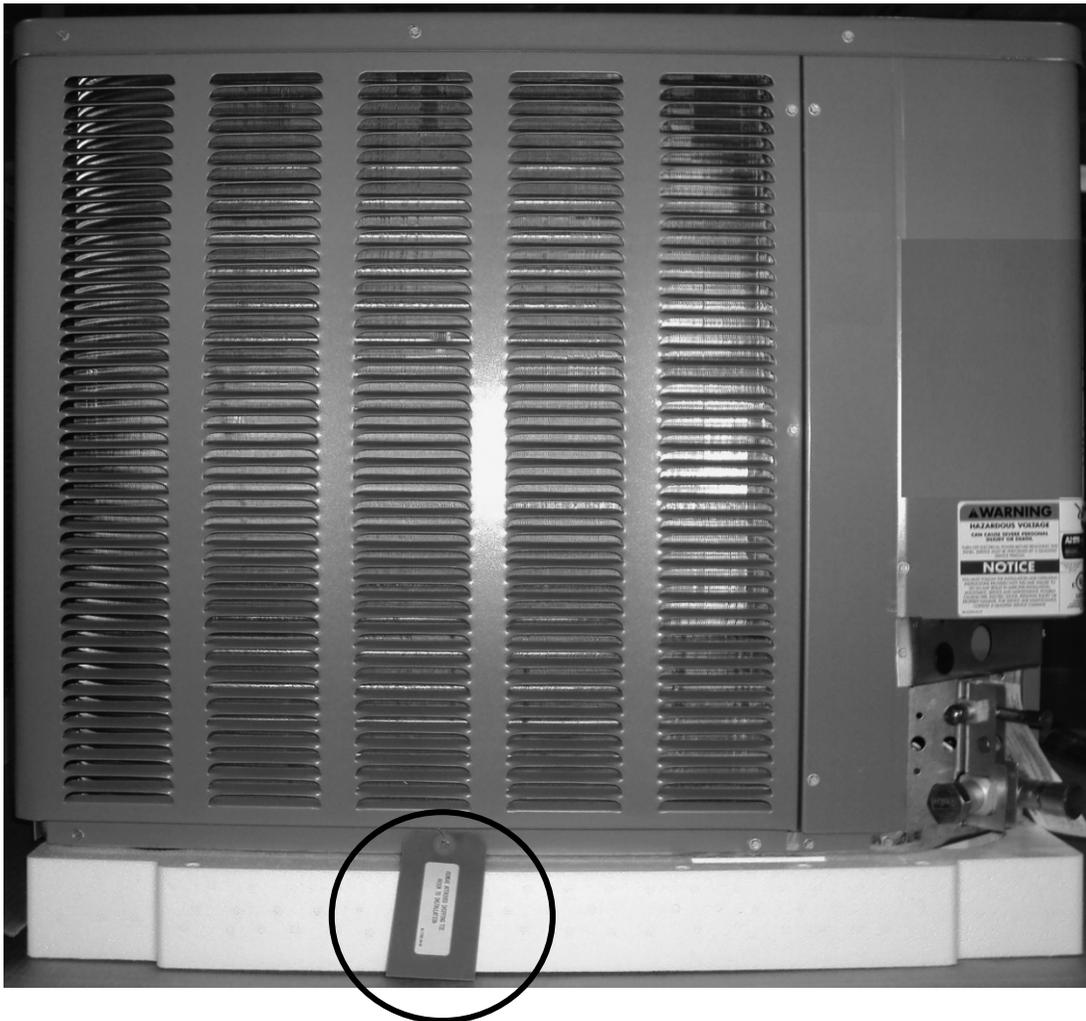
**Notice: Failure to remove strap prior to operation could result in increased internal tubing stress. Plastic strap can be cut off from the exterior of the unit and left inside of the unit.**
