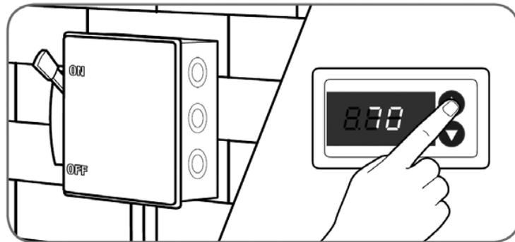
With thermostat in the "Off" position, turn the power on to the furnace or air handler and the heat pump. Start the heat pump and the furnace or air handler with the thermostat.
