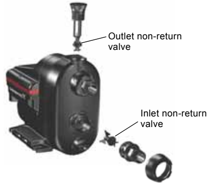
Fig. 21 Outlet and inlet non-return valves
