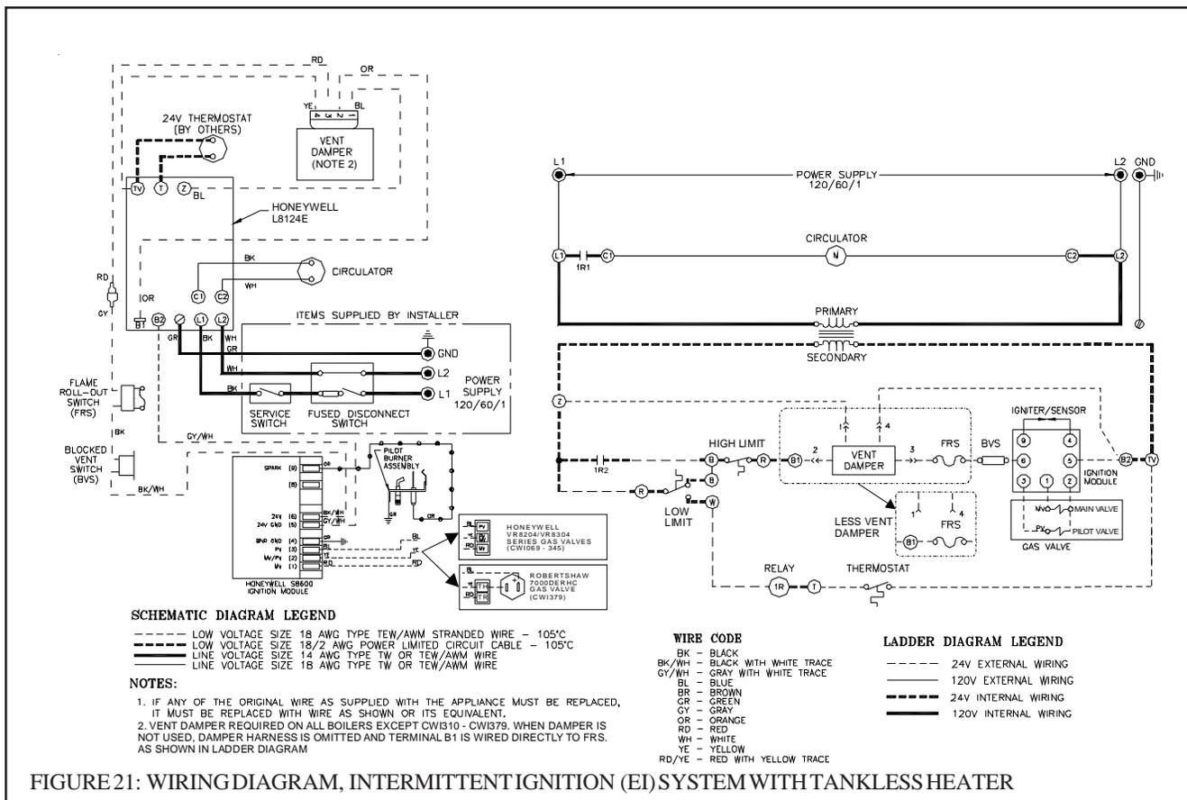
FIGURE 21: WIRING DIAGRAM, INTERMITTENT IGNITION (EI) SYSTEM WITH TANKLESS HEATER
