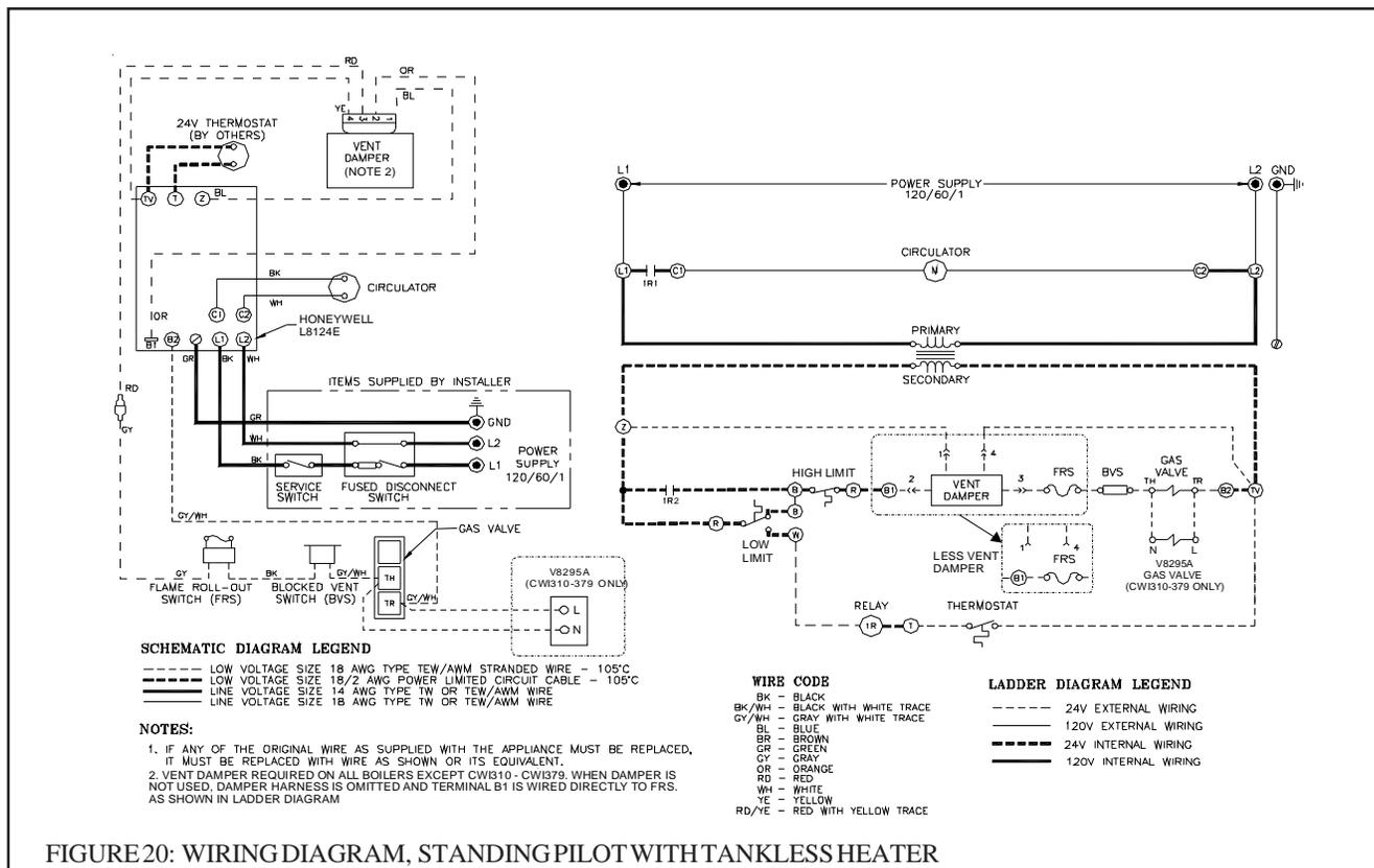
FIGURE 20: WIRING DIAGRAM, STANDING PILOT WITH TANKLESS HEATER
