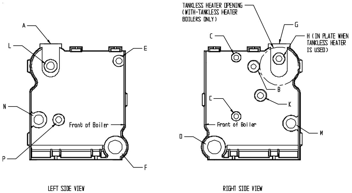
FIGURE A3: TAPPING LOCATIONS (SEE TEXT FOR TAPPING USES)
