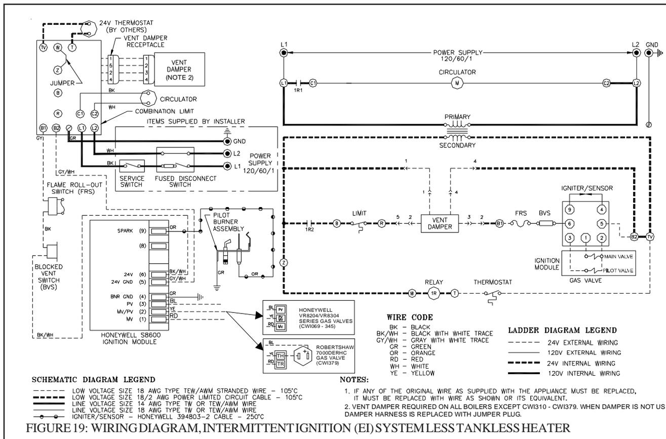
FIGURE 19: WIRING DIAGRAM, INTERMITTENT IGNITION (EI) SYSTEMLESS TANKLESS HEATER
