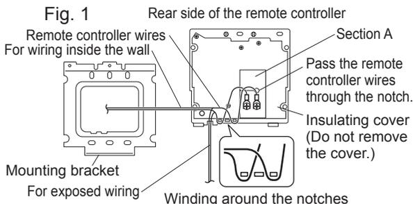
5. Attach the remote controller to the mounting bracket. Insert the bottom of the remote controller into the groove at the bottom of the bracket and push in the 2 hooks on top of the remote controller completely.
