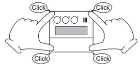
Note: To remove the decorative frame after installation of the remote controller and the frame, pull the entire decorative frame forward while pressing the sections indicated (where the fingers are) in the figure below.
