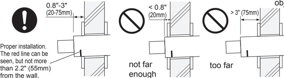
Proper installation. The red line can be seen, but not more than 2.2" (55mm) from the wall.
