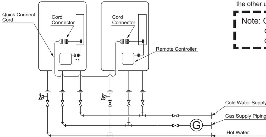
\*1 When connecting two units, disconnect the remote controller connector from the other unit.
