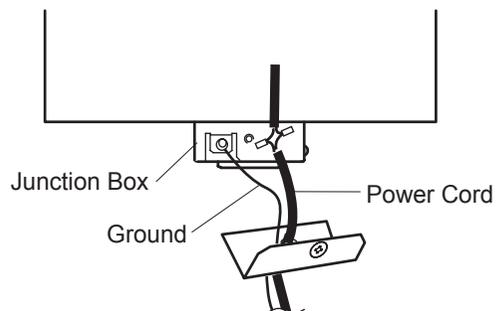
1. Remove the screw (one) of the junction box and open the cover of the junction box.
