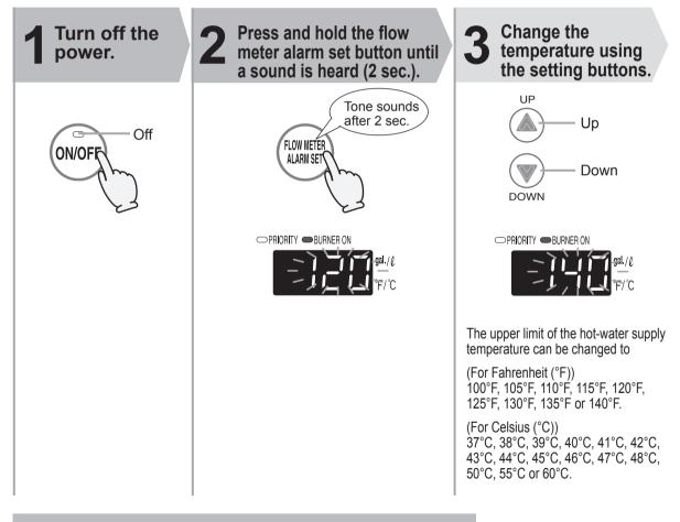
4 Set the Power button to ON when continuing to use the unit as is. Otherwise, let the unit sit for 30 sec.
