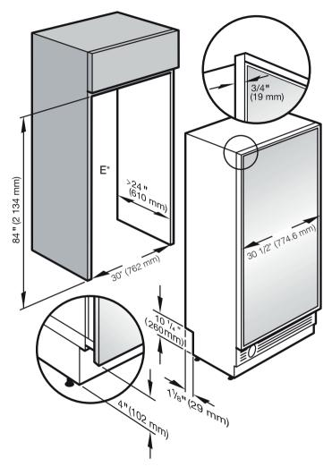
E\*: The position of the electrical connection should not be higher than 9" from the floor.
