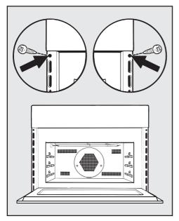
Open the door and use the screws supplied to secure the oven to the side walls of the cabinetry through the holes in the oven trim. Please have the model and serial number of your appliance available before contacting Technical Service.
