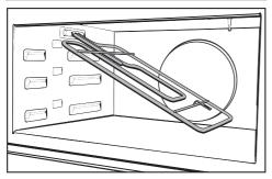
Carefully lower the Browning / Broiling element. The cover at the top of the oven cavity can be damaged. Do not use the hard side of a dish sponge to clean the cover.
