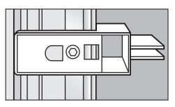
Do not remove the installation supports from the appliance doors. They will be used later in the installation niche.
