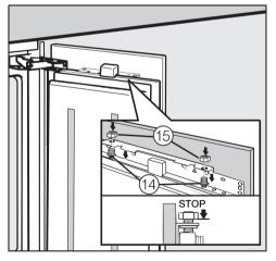
Open the door and hang the custom door with the mounting frame over the threaded bolts (4).
