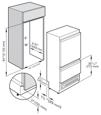
$\mathsf{E}^{\star}:$  The position of the electrical connection should not be higher than 9" from the floor.
