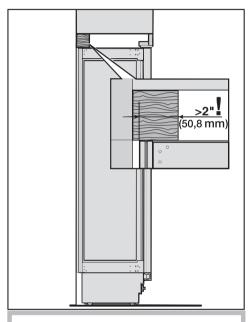
If possible, always screw the wooden beam to existing studs.
