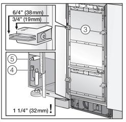
The installation aids ③ on the appliance door have been designed for the following custom door thicknesses:
