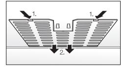
Unhook the filter cover, 1. in each side of the drawer and remove them along with the filter mat downwards starting from 2.
