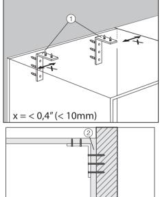
The anti-tip brackets ① keep the appliance safely secured in the installation niche ② and prevent it from tipping.
