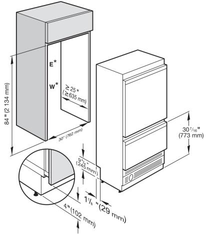
$\mathsf{E}^*:$  The position of the electrical connection should not be higher than 9" from the floor.
